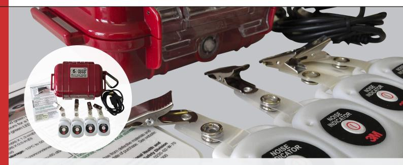
The NI-100 from 3M™ is a simple device to help determine if noise in your work environment is over the OSHA stated threshold of 85 dB. When the badge style unit is turned on and worn by the worker, it flashes green when noise levels are under 85 dB and flashes red when noise is above 85 dB. (+/- 3 dB)
